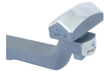
M-132A 50 mm Beginning Low Dome Fluting Stake. The first stake to use for fluting low domed bracelets or cylinders. Use the M-110 Stake for initial forming. This stake prevents misplaced sharp interior marks from forming during the early fluting process.
