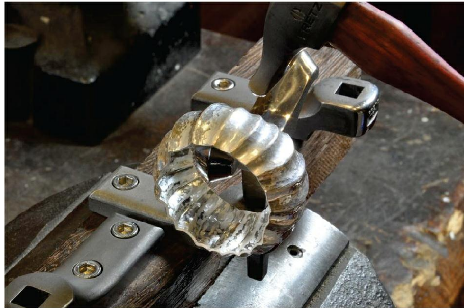
Fluting with the HMR-8 Hammer and Progressive Stakes
