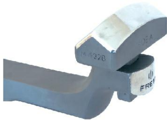
M-132B 50 mm Finishing Low Dome Fluting Stake. The final stake to use for fluting low domed bracelets or cylinders. Use the M-132B to sharpen the flutes formed with the M-132A Stake.
